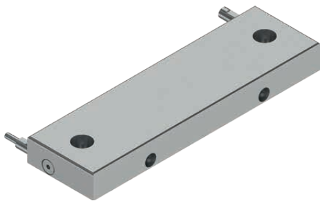
Fig. 6.8 LMFC4-R-IO end block with inlet and outlet holes for connection to the cooling system of the machine at the beginning of the stator track
